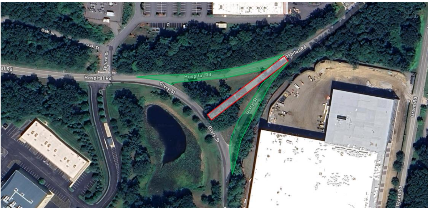
Hospital Givry Street re-alignment project. Green highlighted areas are where pavement has been removed and the red outlined area is the newly aligned road creating a single intersection with Hospital and Givry Streets – August 2025
