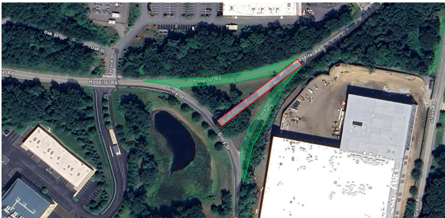
Hospital Givry Street re-alignment project. Green highlighted areas are where pavement has been removed and the red outlined area is the newly aligned road creating a single intersection with Hospital and Givry Streets – August 2025
