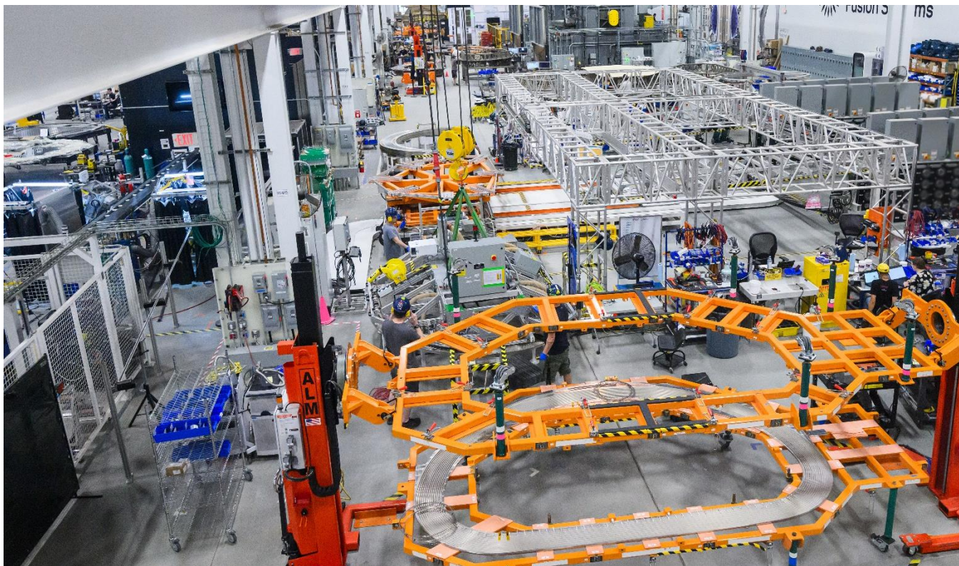
Inside the CFS Magnet Factory at 117 Hospital Road. high-temperature superconducting magnets being assembled to form the magnetic bottle (tokamak) that will contain the fusion process.
