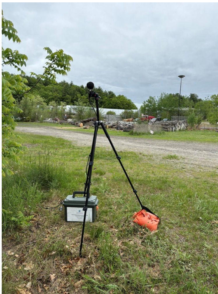
FIGURE 3: Long-Term Sound Monitoring Instrumentation as Installed at the Site.
