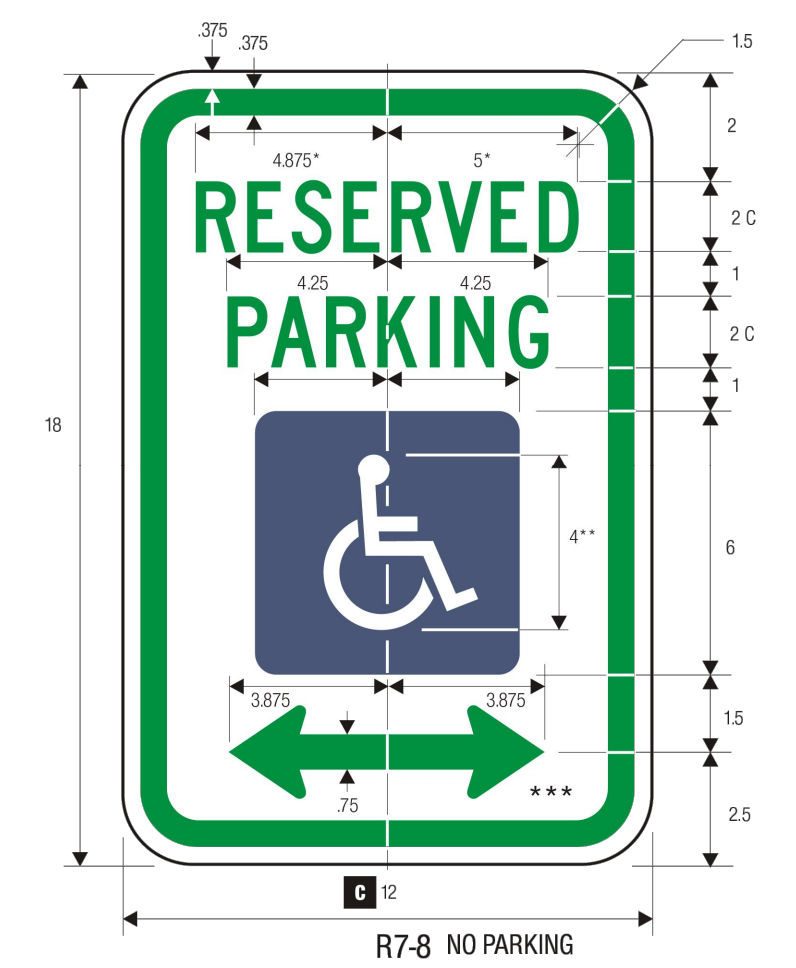
R7-8 NO PARKING LEGEND - GREEN (RETROREFL), WHITE SYMBOL ON BLUE (RETROREFL) BACKGROUND - WHITE (RETROREFL)
