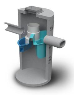
For design purposes the selected model's Treatment Flow Rate must be equal or greater to the site's required Water Quality Flow Rate. The peak flow rate and maximum pipe size must be considered to determine whether an online or offline configuration is appropriate. Full removal curves are available on request.
