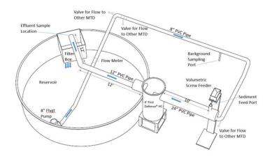
Figure 2 - Set-up of the Portland, Maine hydraulic testing facility
