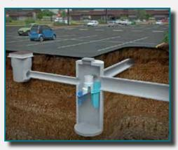
Contaminated stormwater runoff enters the inlet chute from a surface grate and/or inlet pipe. The inlet chute introduces flow into the chamber tangentially to create a low energy vortex flow regime (magenta arrow) that directs sediment into the sump while oils, floating trash and debris rise to the surface.
