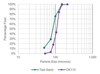
Figure 3 - Particle Size Distribution Comparison
